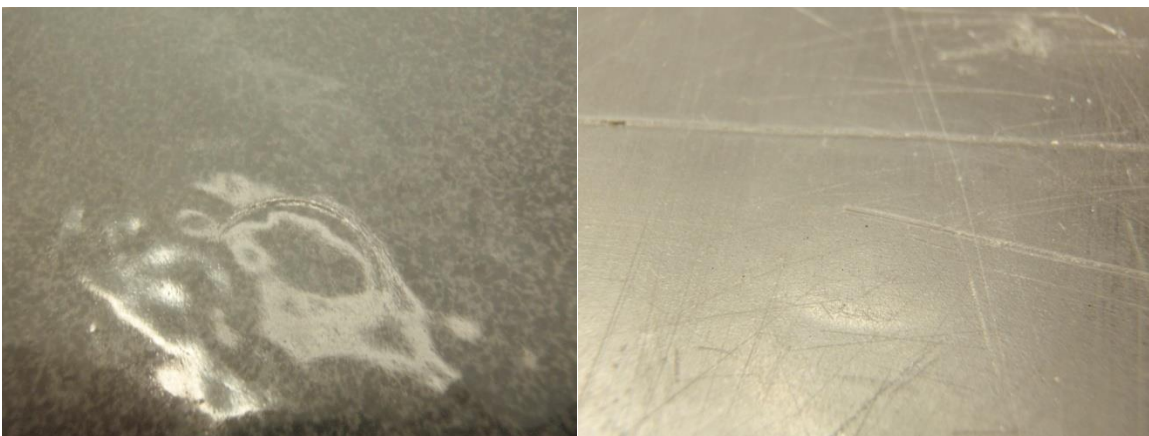
Figure 3: Precidium™ ECS after 320 inch-lb impact
