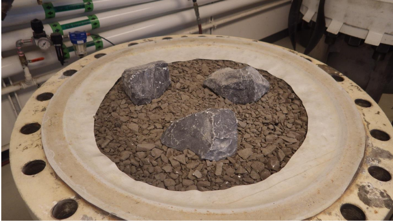
Figure 1: Example of The Subgrade Constructed for the ECS/HDPE Comparison.
