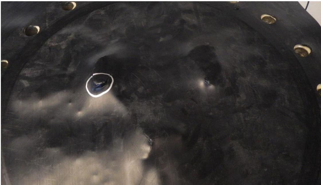
**Figure 3: HDPE Puncture Over 2.5” Gravel Substrate**
