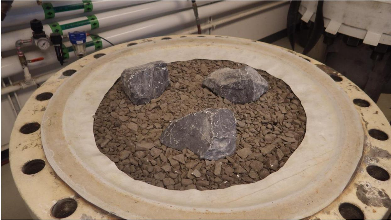
**Figure 1:** Example of The Subgrade Constructed for the ECS™/HDPE Comparison.
