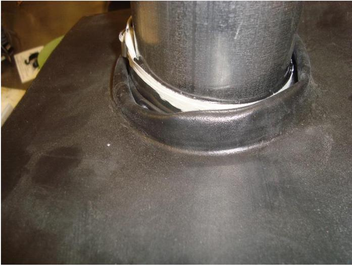
Polyethylene pipe boot pushed upwards to failure
