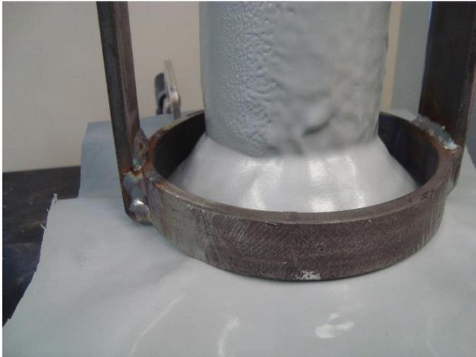
Stretching of Polyurea Boot Prior to Failure
