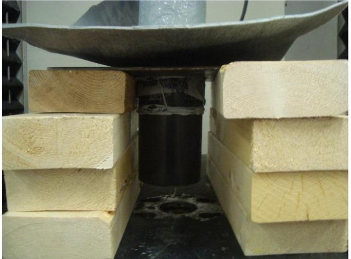
Polyurea connection pushed upwards to failure
