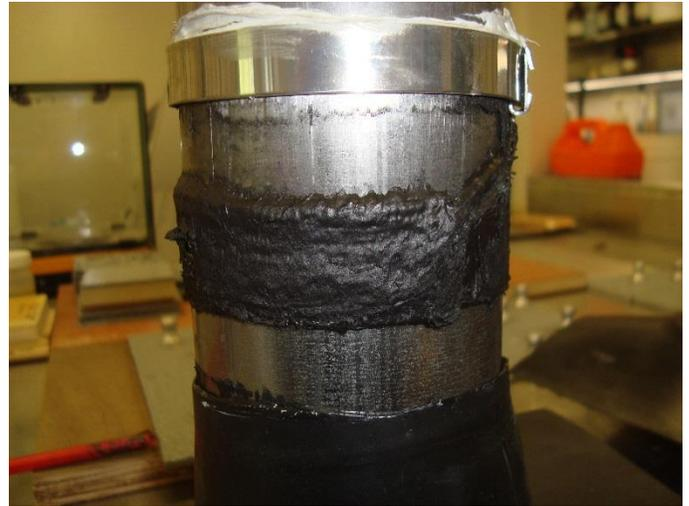
Failure of polyethylene boot Sample 2
