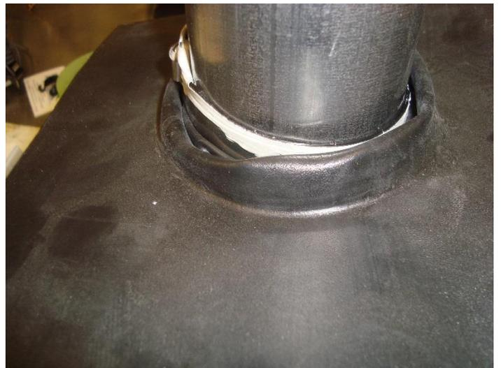
Polyethylene pipe boot pushed upwards to failure
