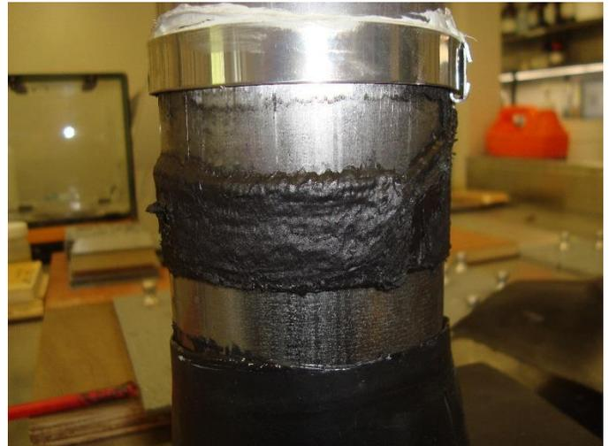
Failure of polyethylene boot Sample 2
